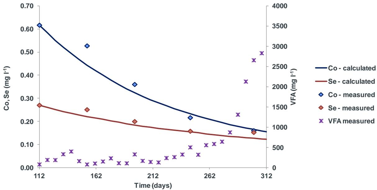
Figure 1 Cobalt and selenium dilute out curves in the pair of digesters where Se, Mo, Co, W, Fe, and Ni supplementation ceased on day 112. (By day 245 the VFA concentration in the digesters had risen above 500 mg l<sup>-1</sup>.)
